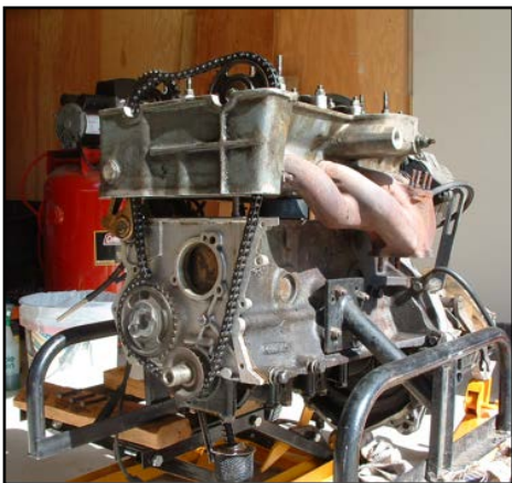
ABOVE: The Lotus Europa Twin Cam water pump is easily replaced... by removing the engine!
